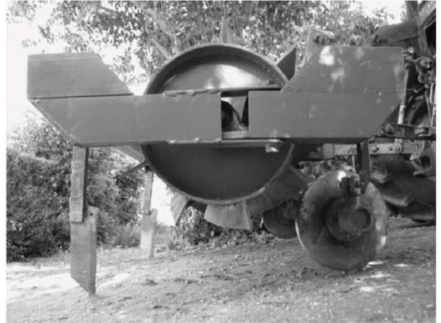
Canali et al. 2013 Fig. 1. Modified roller crimper for transplanting bed preparation (in-line tillage/roller crimper).
